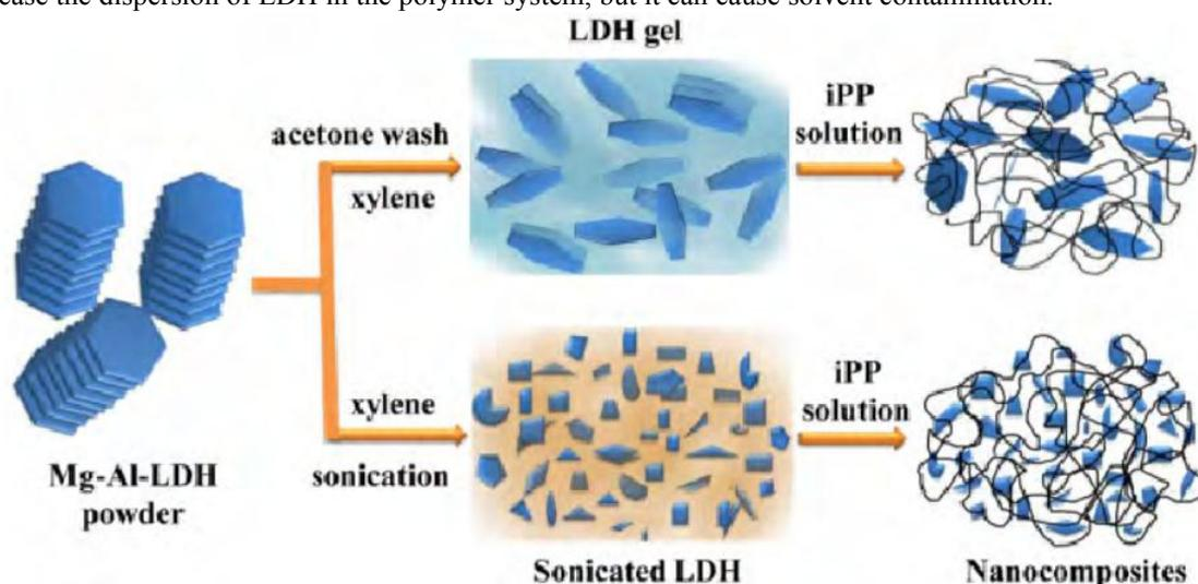
Fig.2 Schematic illustration of iPP/LDH nanocomposite by MgAl-LDH gel and sonicated LDH via solution blending<sup>[31]</sup>
