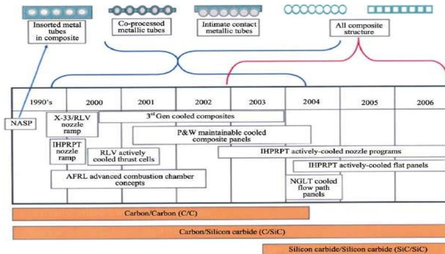
Figure 7 NASA's regenerative cooling ceramic matrix composites
