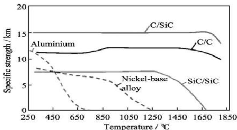
Figure 6 Ratio of strength to weight as a function of temperature
