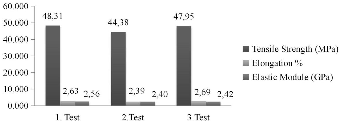
**Figure 2.** Tensile test results
