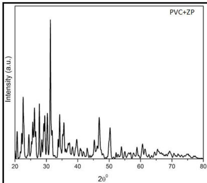
**Figure 4.** Xrd spectra of PVC based ZP composite material
