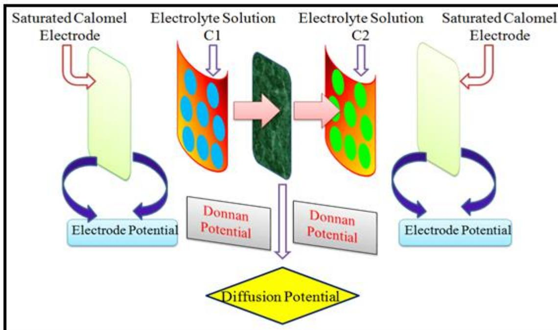
**Figure 1.** Electrochemical setup for ionic potential measurement
