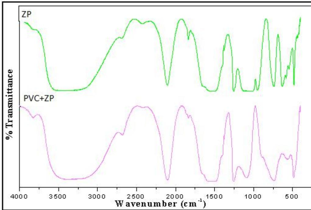
**Figure 3.** FTIR Spectra of only ZP and PVC based ZP composite material
