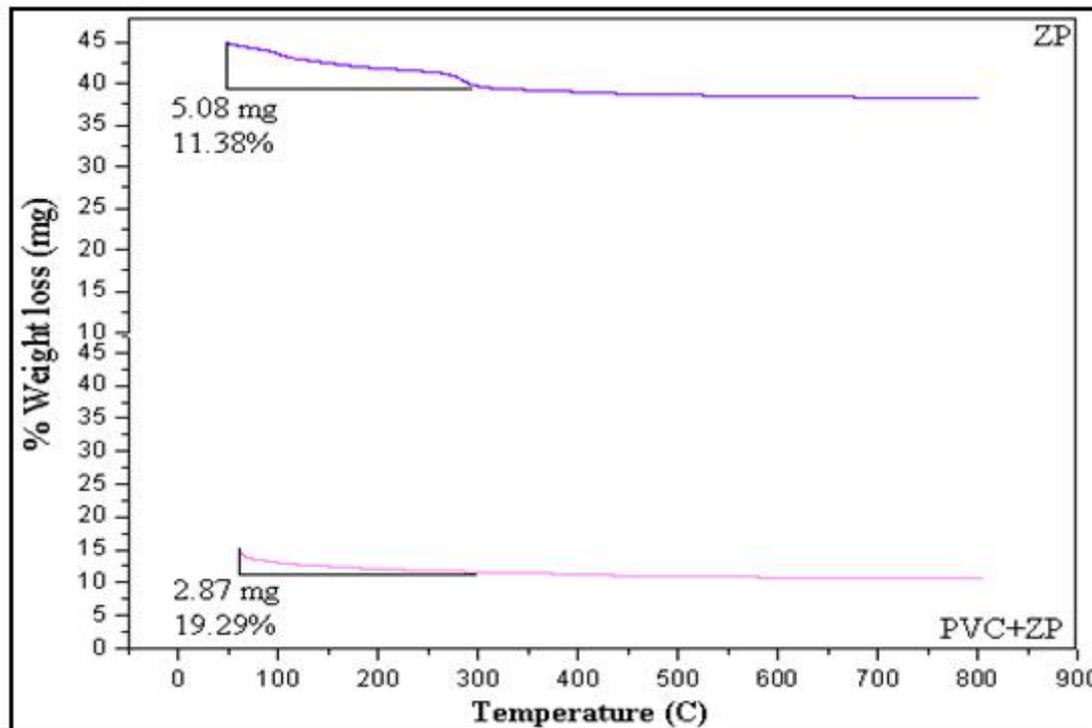
**Figure 5.** TGA spectral analysis of PVC based ZP composite material
