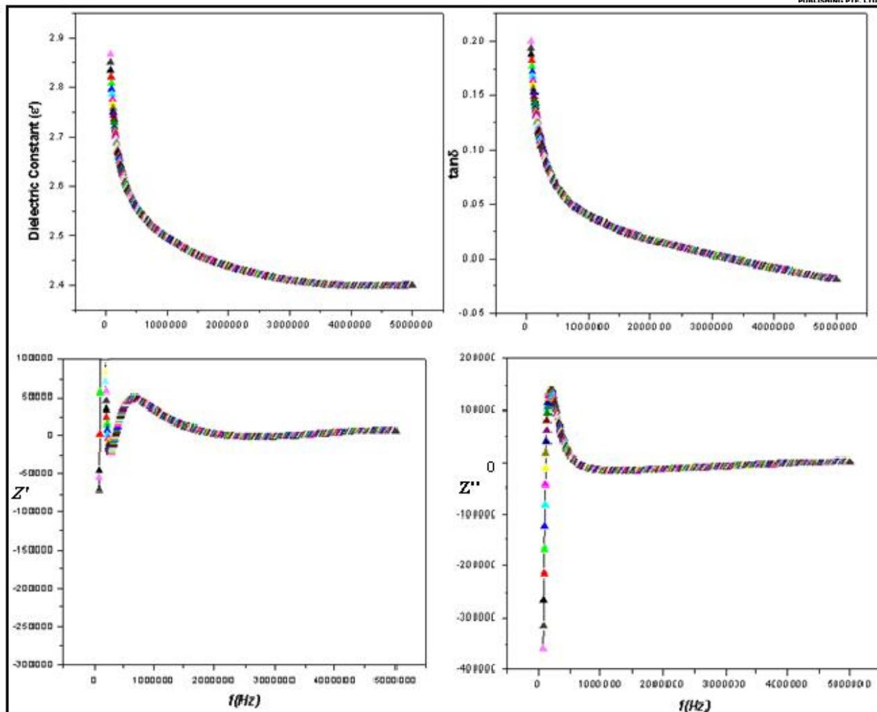
**Figure 6.** Dielectric nature of PVC based ZP composite membrane
