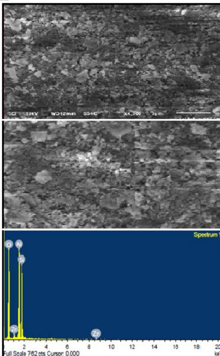
**Figure 2.** SEM supported EDX images of PVC based ZP composite membrane
