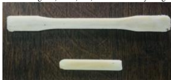
Figure 1. Tensile and impact test specimens
