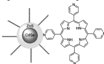
Figure 4; Core-shell structure of CdSe/ZnS quantum dots.
