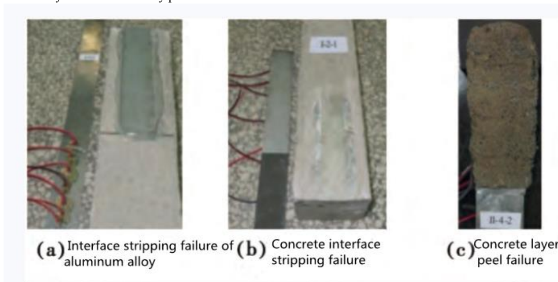
Figure 7; Stripping Failure Form
